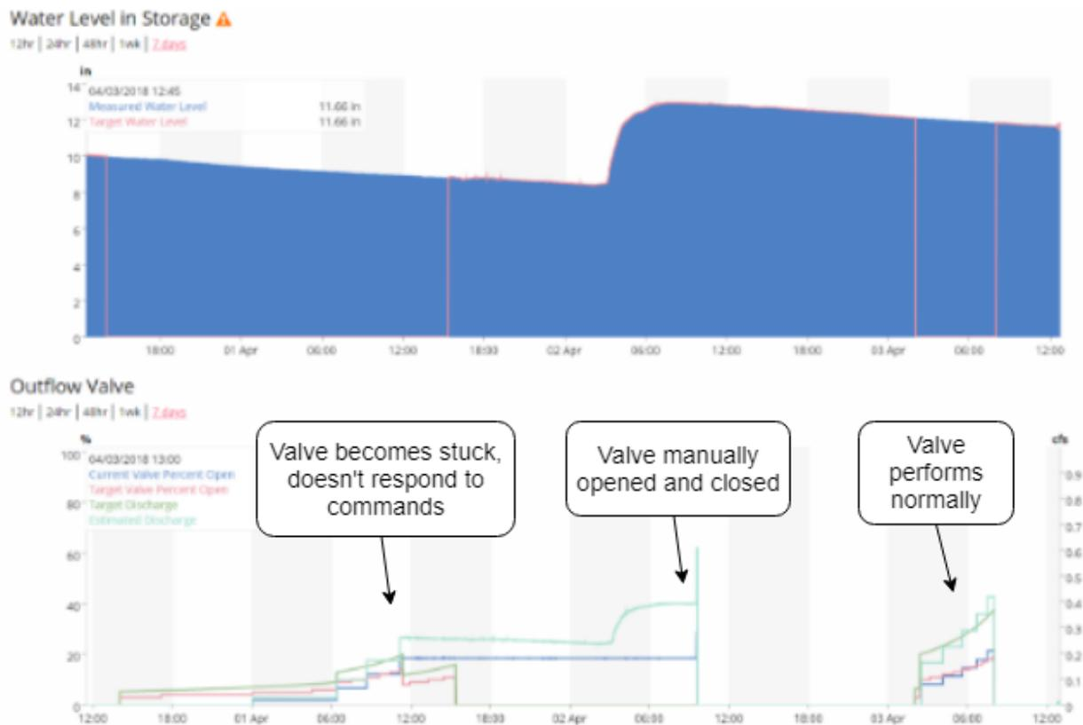
**Figure 8:** Opti dashboard during a valve clog
