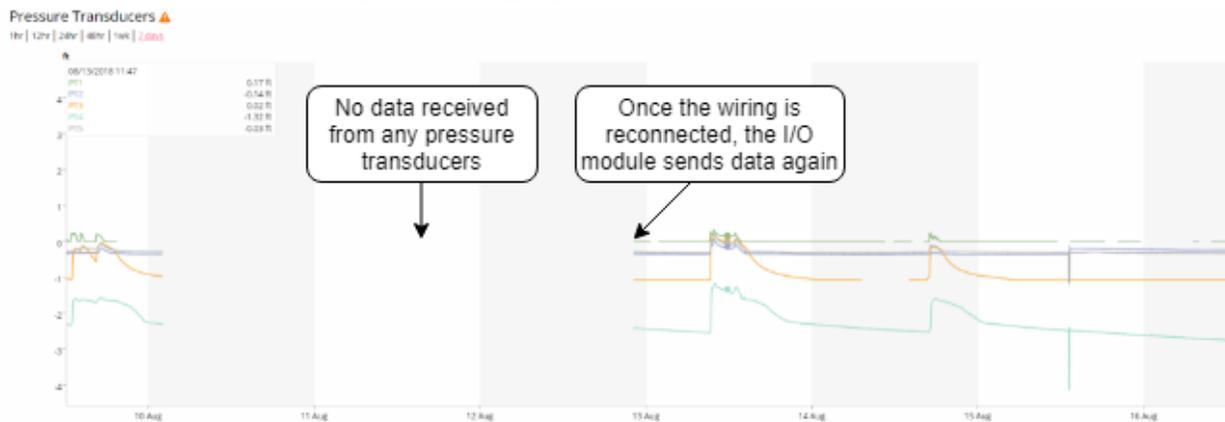
**Figure 10:** Sensor datastream failure during I/O module disconnection
